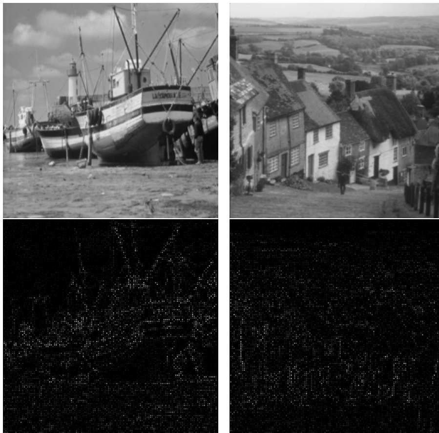
Figure 6: At the top, the images corrected using the Von Neumann neighborhood. At the bottom, the difference, increased ten times, between the reconstructed and the original image.
