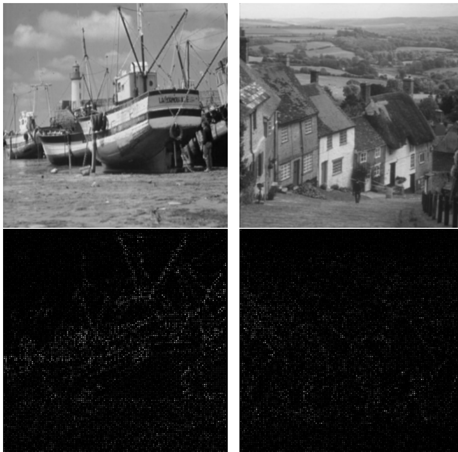
Figure 5: At the top, the images corrected using the Moore neighborhood. At the bottom, the difference, increased ten times, between the reconstructed and the original image.
